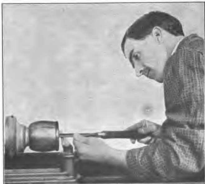
Fig. 189. Working Out the Inside of a Box.
